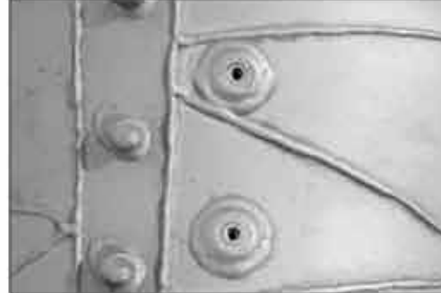
Replaceable fluid ports deliver high pressure fluid stream into the bore, softening the ground and cooling down tooling.
